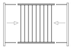
**STEP FIVE:** Drill 16 - 1/8" holes as per diagram and install 3/4" TEK screws to secure gate ends to panel.
