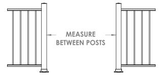
**STEP THREE:** Picket Gate Panel (without Gate End Posts) must be exactly 4.5" less than gate opening. Deduct 4.5" from opening measurement and cut both panel ends, leaving equal picket spacing.
