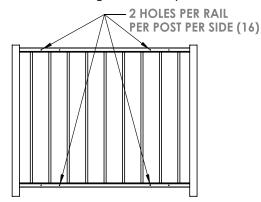
**STEP SIX:** Measure between Gate End Posts, deduct 1/16", cut top/bottom snap covers. Once cut, position snap covers over top/bottom horizontal channels and press in place.
